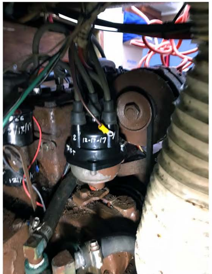
New Ignition Components Installed with dates and cylinder numbers inscribed
