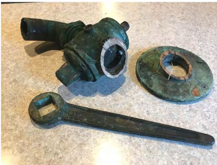
Old Perko valve and through-hull assembly. Note the radial cuts on the through-hull flange to facilitate the removal of the old threaded collar (not pictured). Old valve was frozen stuck in the closed position. Grounding wire (green - see left picture) was attached to the flange with a brass screw. A brass lug was connected and attached with a stainless steel hose clamp to the new valve (not pictured).
