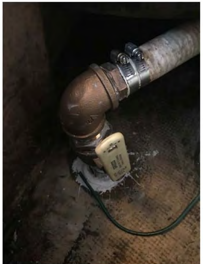
Final through-hull and valve hardware installed to original flexible hose from marine toilet system
